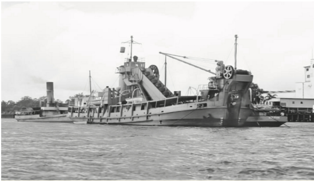
The bucket dredger Groper in the Brisbane River in March 1955. The 738grt Groper was built in 1954 by Fleming & Ferguson at Paisley for the Queensland Government. On 20th July 1981 demolition started on her in Brisbane.
