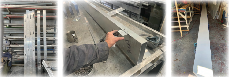
WORK OF DEAN GRAHAM, VEGAS RAILING IN REPLACING ALL THE PRE-EXISTING DAMAGED WHITE TIMBER WITH WHITE POWDER COATED ALUMINIUM
