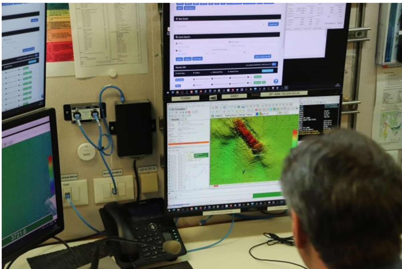
RV Investigator used its advanced multibeam echosounders to create a detailed map of the wreck of SS Nemesis. (Image courtesy: CSIRO/Hugh Barker)
