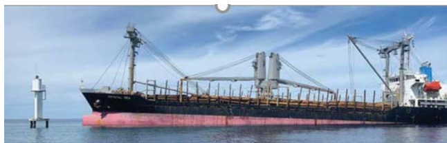
Crystal Sea aground on Greaves Reef - note large stern trim caused through ground reaction under the bow
